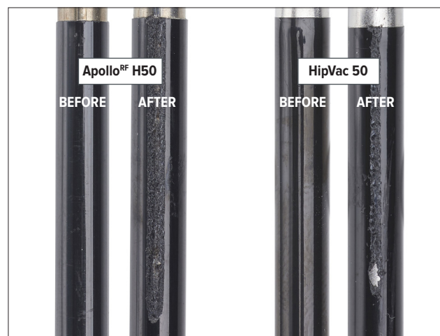
Figure 4. Test samples before and after insulation breach.
