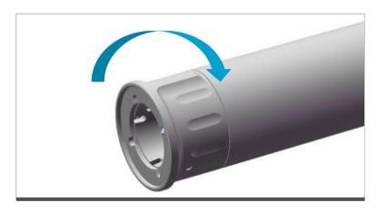
Turn the motor chuck mechanism.
