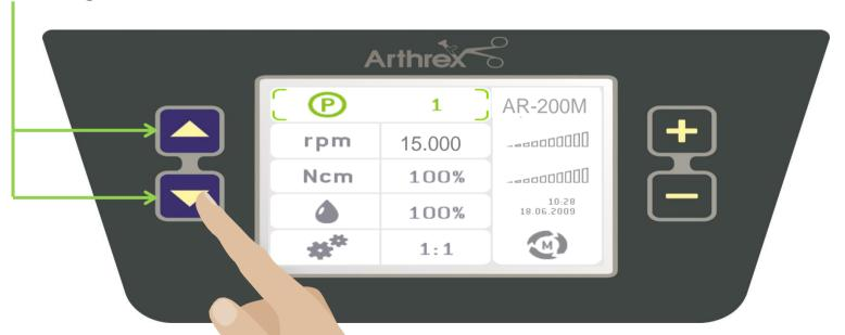
Change speed: Arthrex P AR-200M \_\_\_\_\_ rpm 15.000 Ncm 100% \_\_\_\_\_ 10:28 100% 18.06.2009 1:1
