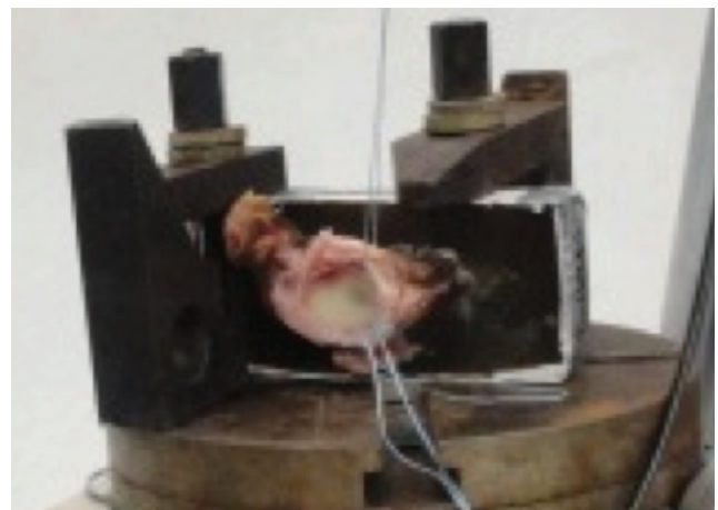
Figure 3. Tissue pull-through test setup
