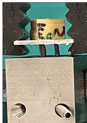
Figure 1A. Test setup with bone blocks and cerclage.
