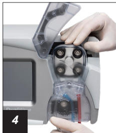
4 *Install outflow cassette
