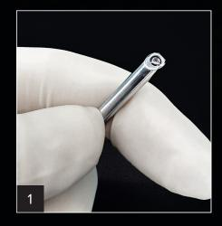
Grasp the distal end of the scope so your index finger is supporting the back side of the scope tip.
