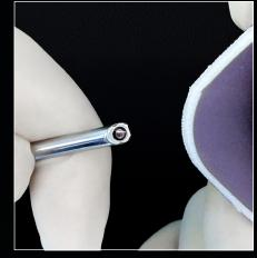
Maintain consistent pressure from the polishing pad onto the distal window of the arthroscope as you "drag" the polishing pad across the window. Repeat 5 to 10 times.
