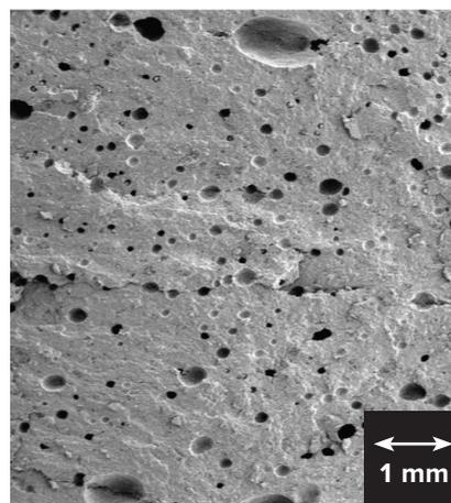
Crystallization process completed showing presence of porosity
