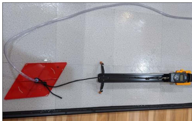
Figure 3. Setup for Resistance to Movement Test
