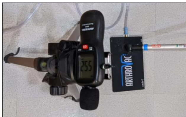
Figure 3. Setup for Resistance to Movement Test
