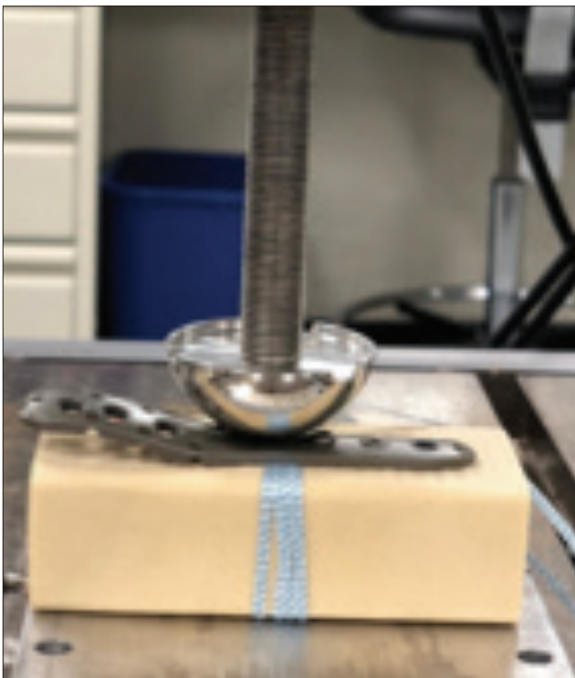
Figure 1. Setup for dynamic compression (fatigue) test to investigate suture damage and fraying.
