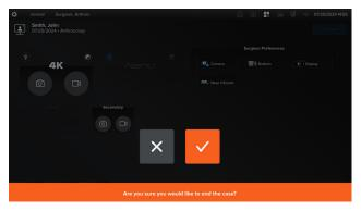
When you are ready to end the case, press the blue End Case button at the upper-right corner and confirm your selection by clicking the check mark.
