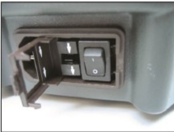
Figure 6-11 Fuse Replacement: Slide Out Holders
